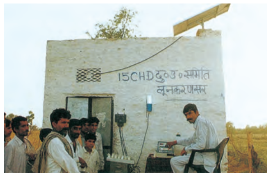
Fig. 5.10: Solar operated electronic milk testing equipment
